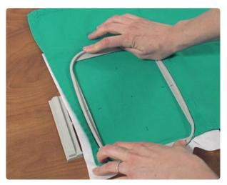
Hoop the napkin with a piece of cutaway stabilizer. Line up the marks on the napkin with the marks on the hoop.
