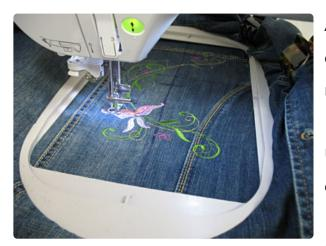
Attach the hoop to the machine and load the design. Move the hoop so that the needle is right over the center point.
