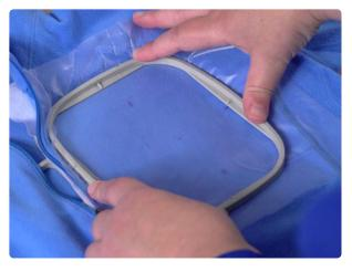
Hoop all three layers together -- stabilizer, fleece, and topping. Hooping all three layers together guards against shifting and gaps in the stitchout.
