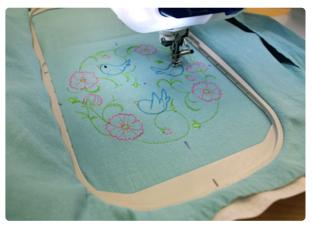
Use a size 11 or 75/11 sharp sewing needle. A sharp sewing needle has a smaller, finer point than an embroidery needle, so it will make the smallest holes in the tear-away stabilizer. That helps guard against shifting and misaligned stitches.
