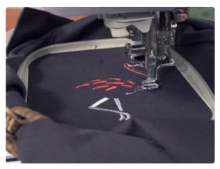
Attach the hoop to the machine and load the design.
