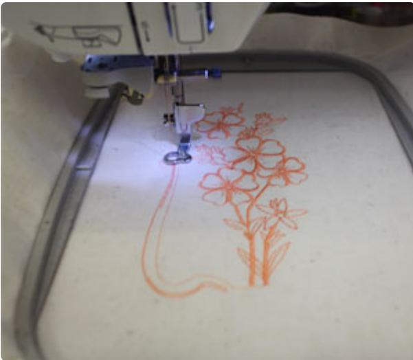
As muslin is a loose-weave fabric, using a light- or medium-weight cutaway stabilizer (1.5 - 2.5 ounce) is the best way to ensure crisp-looking results. Hoop the fabric and stabilizer together for crisp, neat, and clean stitches.
