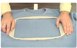
Then, when you're hooping the fabric and stabilizer, you can line up the horizontal and vertical axis lines with the markings on the hoop.
