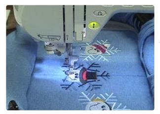
Attach the hoop to the machine and move the hoop so that the needle is right over that center point; then embroider the design.
