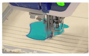
Attach the hoop to the machine, and continue embroidering the design. The next stitch is a tackdown, or zigzag stitch, and that binds the applique fabric to the towel.
