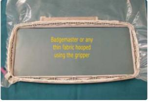
In this photo, the hooping is complete, with a water-soluble stabilizer. See how nice and tight the stabilizer is? And the really great thing is that it will not slip as the design stitches!
