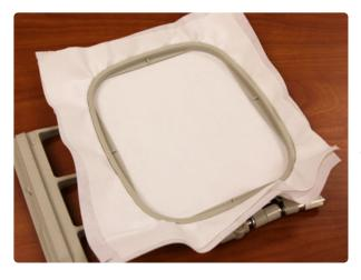
Hoop the fabric or item with one piece of cutaway stabilizer.
