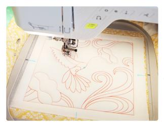
Load the embroidery file onto the machine, and move the needle until it is above the marked center point. Then embroider the design.
