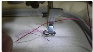
Adjust the thread tension to account for the thick thread. The "normal" tension on embroidery machines is set for 40 weight thread. Because the 12 weight is much thicker, you may find that you need to loosen the upper thread tension. I opened the upper thread tension plates as much as possible; you may find that you get good results with a lesser degree of change.
