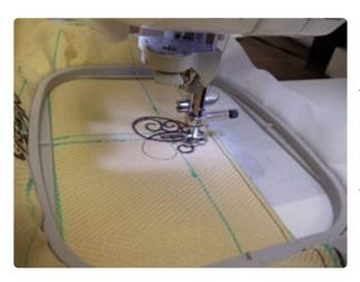
Attach the hoop to the machine and load the design. Move the hoop so that the needle is directly over the center point on the fabric. Embroider the design.
