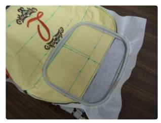
Spray your stabilizer with a bit of temporary adhesive, and smooth the fabric on top. Hoop the fabric and stabilizer together by aligning the marks on the hoop with the lines on the fabric.
