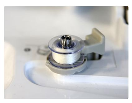
Freestanding lace is seen from both sides, so wind a bobbin with the same thread that you're using in the needle.
