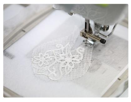
Attach the hoop to the machine and load file "a". In this example, 40 weight rayon thread was used. You can also use 30 weight cotton or metallic thread for most freestanding lace designs.
