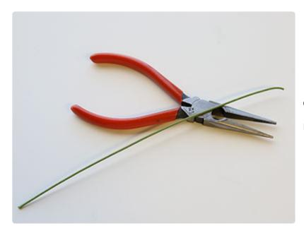
Cut the wire to 10" long with a needle nose pliers or wire cutter.
