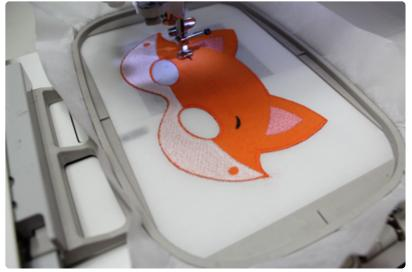
Other elements of the design will sew. Watch for a note on the color change sheet that says "back piece tackdown". When you reach this step, remove the hoop from the machine and turn it over to the backside.
