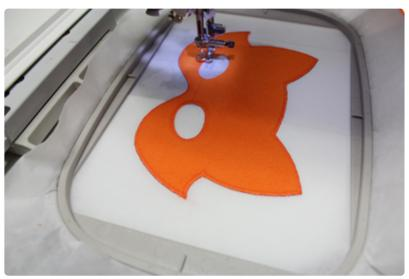
Attach the hoop back onto the machine and continue with the design. A tackdown stitch, also called a zigzag stitch, will sew next. This will bind the fabric to the stabilizer.
