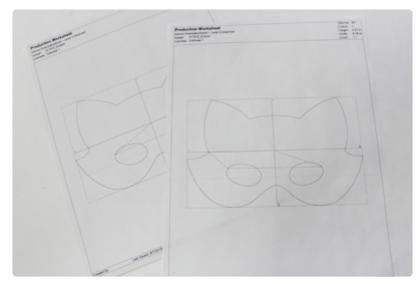
Download the mask design and unzip it. Extract the files and look for those marked with the letters "DL". Those files are the dielines. Dielines are used to cut fabric to the right shape and size of the masks. Print the dielines; if you don't have embroidery software, Wilcom's TrueSizer is a free program that can print templates.
