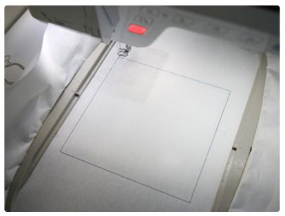
Use a size 11 or 75/11 sharp sewing needle, rather than an embroidery needle. A sharp sewing needle has a smaller, finer point than an embroidery needle, so that will make smaller perforations in the stabilizer.
