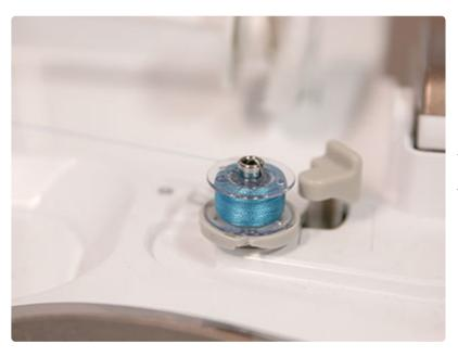
Since both sides of the mug rug will be seen, wind a bobbin with the same thread used in the needle.
