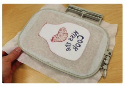
Remove the hoop from the machine -- but don't take the stabilizer out of the hoop. Instead, turn the hoop over.
