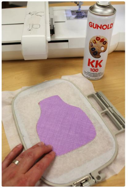
Spray the stabilizer side of the back piece fabric with a bit of temporary adhesive. Then, place it on the back of the tear-away stabilizer.
