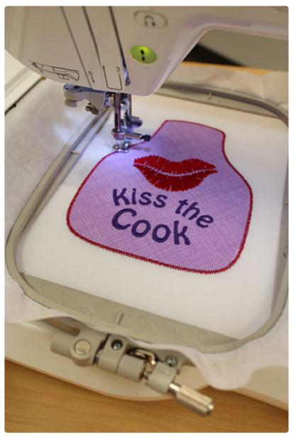
Attach the hoop to the machine, and continue embroidering the design. The tackdown stitch will sew, which binds the back fabric to the stabilizer. Then, a border and buttonholes will sew.
