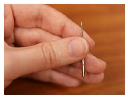
Use a size 11 sharp sewing needle in the machine rather than an embroidery needle. A sharp sewing needle is the best choice when embroidering in-the-hoop designs.
