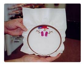
Rehoop the fabric, and load the bottom section into the embroidery machine. The bottom section will begin at the center of the top of the design. Position the needle so that the bottom overlaps the midsection by about one-quarter inch.
