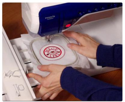
Attach the hoop back to the machine. Continue the design.
