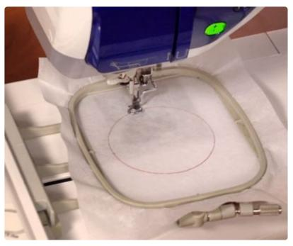
Attach the hoop to the machine and load the full embroidery file (not the DL files).
