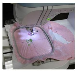
Attach the hoop to the machine, and load the design. Move the hoop so the needle is directly over the center point on the fabric, and embroider the design.
