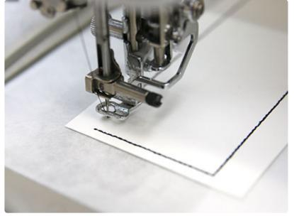
Next, place the hoop back on the machine and embroider the "Cut line." This marks the area on the paper piece where the finished design will later be cut out. It also holds the paper piece in place.
