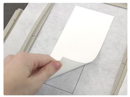
After the dieline has sewn, remove the hoop from the machine but do not unhoop the stabilizer.
