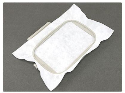
Hoop a piece of medium-weight cutaway stabilizer. Make sure it is tight in the hoop with no wrinkles.
