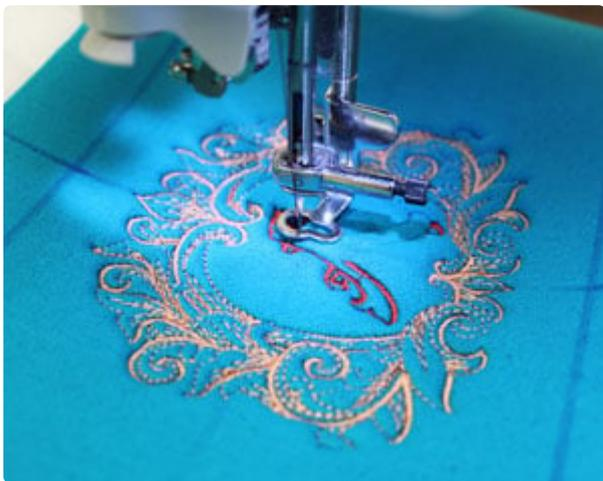
Attach the hoop to the machine and load the design. Move the hoop so that the needle is directly over the center point on the fabric and embroider the design.
