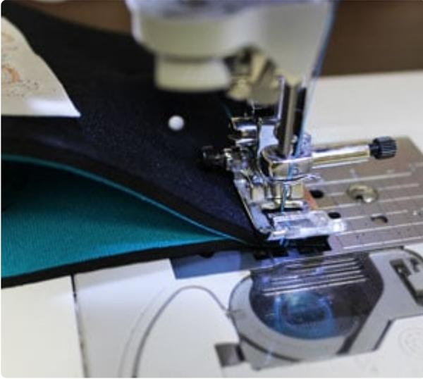
Sometimes the double layer of neoprene gets too thick for the machine to properly form a stitch. If this occurs, you can try slowing your machine down to its lowest setting. Or, glue the seam by simply adding fabric glue along one short end, align the short ends together, and press in place.
