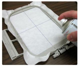
Hoop the stabilizer by aligning the marks on the hoop with the lines on the stabilizer. Spray the stabilizer with temporary adhesive.
