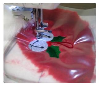
Attach the hoop to the machine, load the design, and align the needle over the center point you marked on the tape. Remove the tape and add a piece of heavy weight, water-soluble stabilizer over the fabric, and embroider the design.
