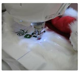
Attach the hoop to the machine and load the design. Align the needle over the center point on the tape. Remove the tape and then lay a piece of heavy weight, water-soluble stabilizer over the fur trim and embroider the design.
