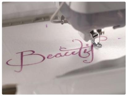
Attach the hoop to the machine, and load the design. Move the hoop so that the needle is right over the center point, and embroider the design.
