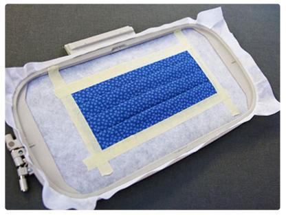
Make sure the pleats are opening toward the bottom edge of the dieline, especially if you are rotating the file. This way the machine will sew the pleats down in the correct direction, preventing them from getting caught on the machine hoop.
