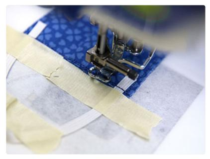
Return the hoop to the machine and embroider the elastic tackdown. This will sew the ends of the elastic or ties in place.
