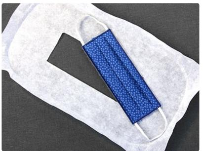
Once the finishing boarder is finished, unhoop the stabilizer and remove the excess from around the face mask. If using water soluble stabilizer, make sure to trim away as much stabilizer as you can, and wash your mask in a washing machine to remove any remaining stabilizer.
