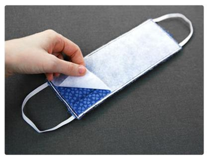
For tearaway stabilizer, also tear off the remaining stabilizer from the backside of the face mask. After this is torn away, no stabilizer should be visible, and the fabric mask should be soft and flexible.
