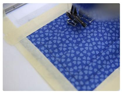
Place the hoop back onto the machine and embroider the tackdown for the face mask. The tackdown holds the fabric in place for the remainder of the design.
