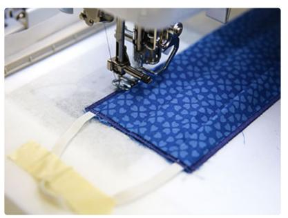
Remove any tape that is on or near the fabric, but make sure the loop is still taped down to the stabilizer. Place the hoop back on the machine and embroider the finishing border. This will sew the final border around all four edges of the fabric.
