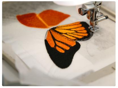
Attach the hoop back onto the machine and continue with the design. At each color stop, match the bobbin thread to the top thread and continue with the design.
