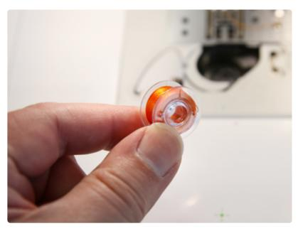
When the machine stops for each color, remove the hoop but do not unhoop the stabilizer. Change the bobbin to match the next color.
