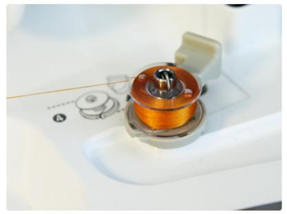
To start, wind a bobbin for each color of the design. The back of the design can be seen, so match the bobbin thread to the top thread (the thread in the needle).
