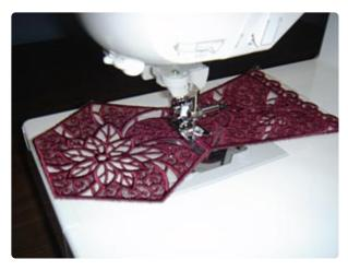
Lay the base hexagon piece right side up. Align the short side of a side piece, wrong side up, with the edge of the base. Using a matching thread color and a zig-zag stitch, sew the pieces together.
