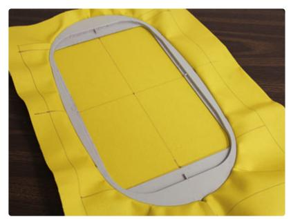
Remove the template. Hoop the fabric and stabilizer together, aligning the marks on the hoop with the marks on the fabric. Attach the hoop to the machine and load the design. Move the hoop so that the needle is aligned with the center point on the fabric. Embroider the design.
