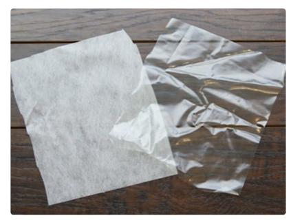
There are a couple of different kinds of heavy-weight, watersoluble stabilizer. One is clear and plastic, and that brand is Sulky Ultra Solvy. The other is soft and fibrous, called Vilene. Both will work very well. Sulky Ultra Solvy is used in this demonstration.
