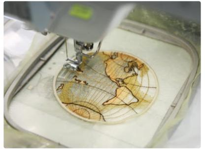
Load the design onto the machine, and embroider the globe.
