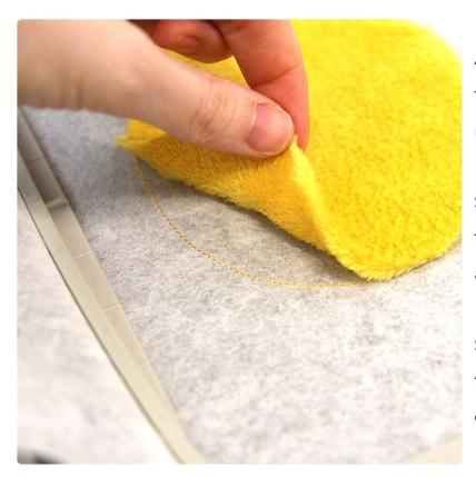
After the dieline has sewn, remove the hoop from the machine, but do not unhoop the stabilizer.
