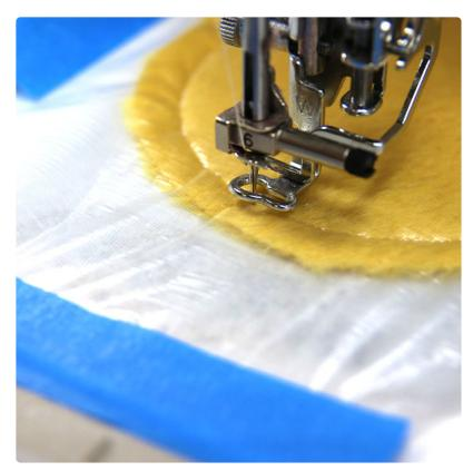
Place the hoop back onto the machine and embroider the tackdown for the front fabric piece. The tackdown will hold the fabric piece in place for the remainder of the design.
