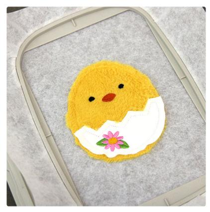
Once all the inner details are done embroidering, remove the hoop from the machine, but do not unhoop the stabilizer.
