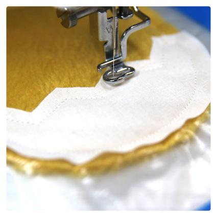
Return the hoop to the machine and stitch out the "Applique tackdown" step.
