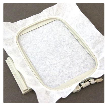
Hoop a piece of tear-away stabilizer firmly. Make sure it is nice and taut with no wrinkles.
