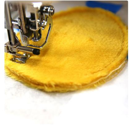
Place the hoop back onto the machine and embroider the back piece tackdown. This will adhere the front and back pieces together. It will also leave a small opening along the edge for turning.
