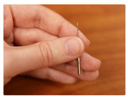
Use a size 11 sharp sewing needle in the machine rather than an embroidery needle.
