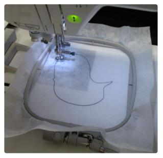
Attach the hoop to the machine, load the design (the file that starts with "X" followed by 4 numbers) and begin embroidering the holder.
