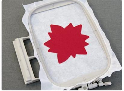
After the dieline has sewn, remove the hoop from the machine, but do not unhoop the stabilizer. Spray the stabilizer side of the front fabric piece with temporary adhesive.
