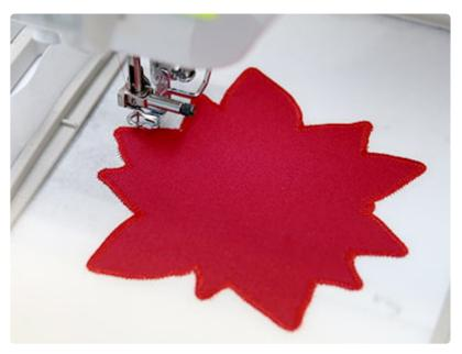
Then place the hoop back onto the machine, and embroider the tackdown for the front fabric piece.
