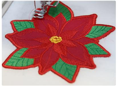
Place the bobbin into the machine, and follow the color change sheet to embroider the remaining "back piece tackdown" and "finishing border" steps.
