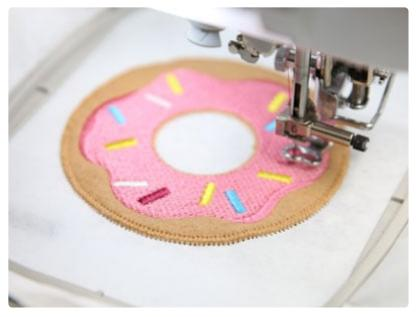
Attach the hoop back onto the machine and continue with the design.
