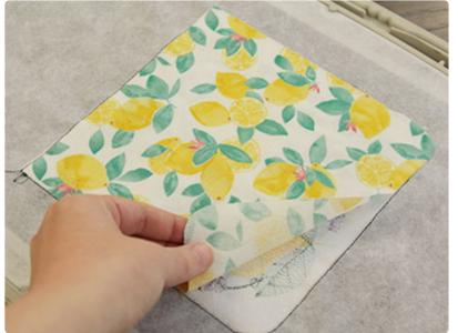
Before sewing the "pocket lining tackdown" step, remove the hoop from the machine, and turn it over so the back side of the embroidery is facing up. Then spray the back side of the pocket lining piece with temporary adhesive and smooth it into place on the back side of the embroidery.
