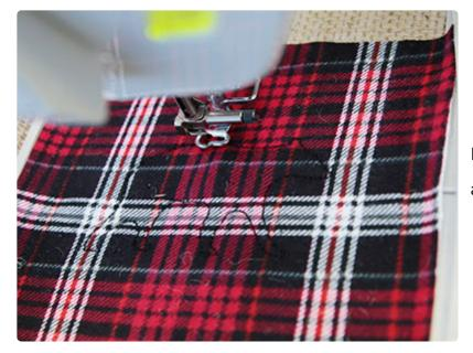
Return the hoop to the machine and sew out the front tackdown.
