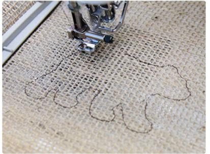
Attach the hoop to the machine and load the file. Begin to embroider the design. The first thing to sew out will be the "outline". This marks the area on the burlap to help with placement of the hanger.
