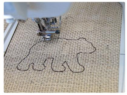
Now sew out the "back piece tackdown". Don't worry if it sews over the tape; the tape can easily be torn away from around the stitches.
