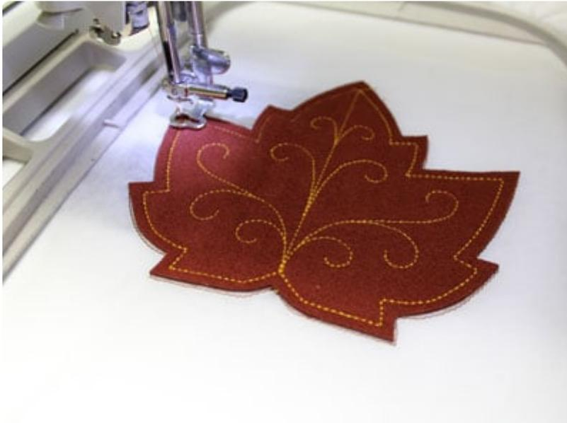
Attach the hoop back to the machine. Continue the design.
