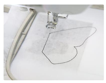
Use a 11 (or 75/11) sharp sewing needle instead of an embroidery needle. A sharp sewing needle has a smaller, finer point than an embroidery needle, so it will make smaller perforations in the stabilizer.
