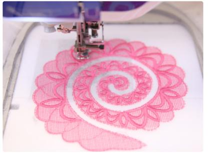
Attach the hoop to the machine, load the file, and embroider the design.
