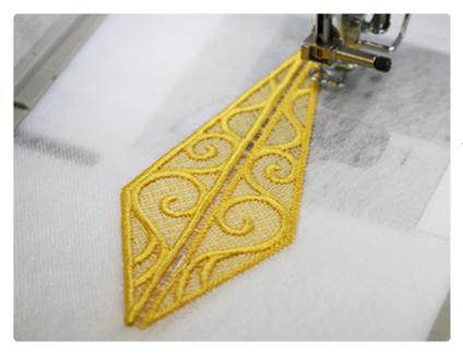
Attach the hoop to the machine and load file "a". Embroider the design.
