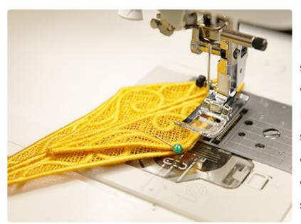
Make sure to use a matching bobbin when sewing. Using a sewing machine, sew a 3.5mm wide zigzag stitch and sew the two pieces together along one short side. Sew around the satin border of the pieces, so the needle "falls off" one side of the lace piece while sewing.
