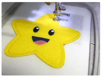
Attach the hoop back onto the machine and continue with the design. A running stitch tack down will sew -- this binds all the layers together.
