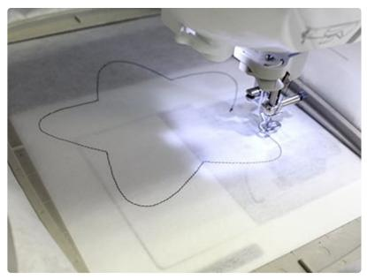
Use a size 11 or 75/11 sharp sewing needle, rather than an embroidery needle. A sharp sewing needle has a smaller, finer point than an embroidery needle, so that will make smaller perforations in the stabilizer.
