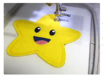
Attach the hoop back onto the machine and continue with the design. A running stitch tack down will sew -- this binds all the layers together.
