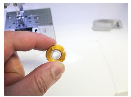
The remaining steps will be seen from both sides. Wind a bobbin with the same thread used in the top.
