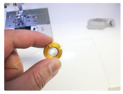
The remaining steps will be seen from both sides. Wind a bobbin with the same thread used in the top.
