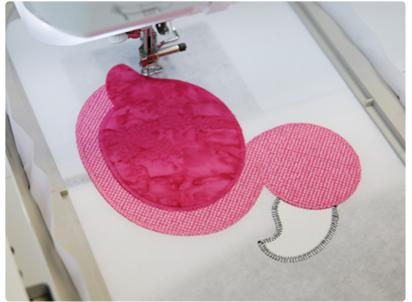
Repeat again to remove the hoop from the machine, spray the wrong side of the fabric piece, place it inside the sewn dieline, and embroider the tackdown step.
