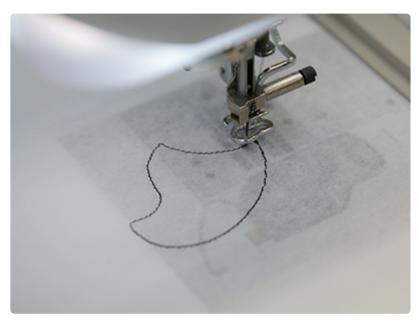
Attach the hoop onto the machine, and load the embroidery file (not the dieline files).
