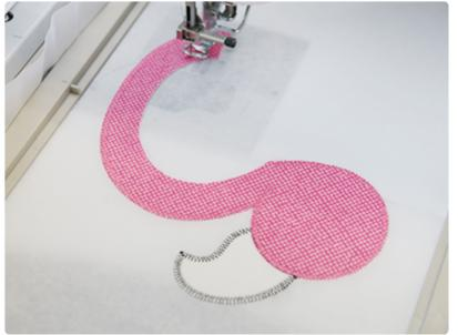
Repeat to remove the hoop from the machine, spray the wrong side of the next fabric piece, and smooth it inside the sewn dieline. Then embroider the tackdown step.
