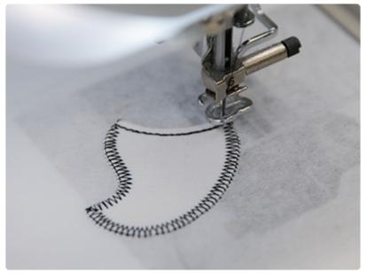
Then place the hoop back onto the machine, and embroider the tackdown for the fabric piece. The tackdown will hold the fabric piece in place for the remainder of the design.
