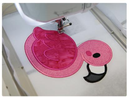
Place the bobbin into the machine, and follow the color change sheet to embroider the rest of the design.
