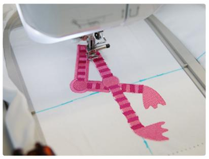
Load the embroidery file onto the machine, and secure the hoop in place. Then move the needle directly over the marked center point on the towel.
