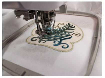
Then, the inside detail will stitch. In this example, the ferns are sewing.
