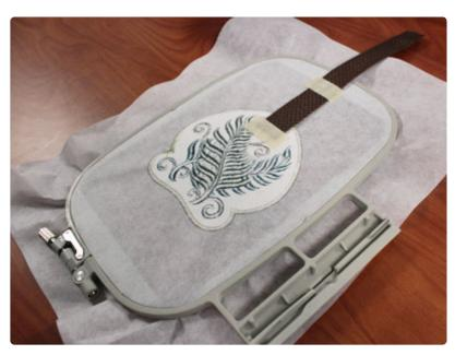
On the color change sheet, look for the note that says "back piece tack down." When you get to this step, stop the machine, remove the hoop, and turn it over.
