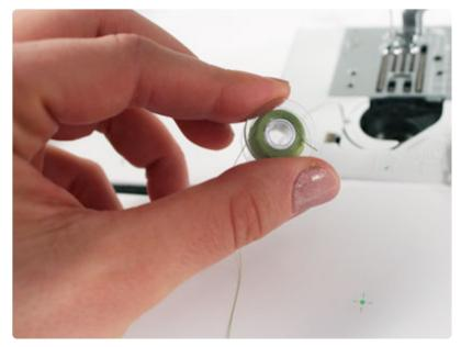
The rest of the design will be seen from both sides. Wind a bobbin with the same thread that you're using in the needle.
