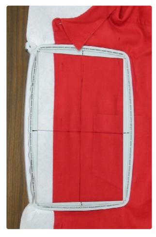
Front placket designs: Use a small amount of spray adhesive to affix the shirt front to the stabilizer. Extend the horizontal axis line onto the stabilizer, and hoop the combination together, lining up the axis lines with the center markings on each side of the hoop.
