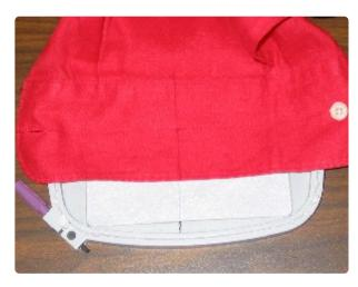
For the cuff design, hoop the stabilizer and mark the stabilizer with axis lines between the center markings on the sides of the hoop. Spray the stabilizer with spray adhesive and match up the marked lines on the cuff with the lines that you marked on the stabilizer.
