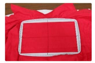
Hoop the back yoke together with stabilizer. Match up the axis markings on the shirt with the center marks on the sides of the hoop.
