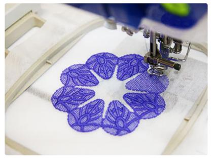
Attach the hoop to the machine and load file "a". Embroider the first piece using a matching bobbin.
