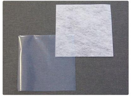
There are a couple of different kinds of water-soluble stabilizer. One is clear and plastic, and that brand is Sulky Ultra Solvy. The other is soft and fibrous, called Vilene. Both work very well. Vilene is used in this demonstration. Use a size 11 or 75/11 sharp sewing needle. A sharp sewing needle has a smaller, finer point than an embroidery needle. That means it will make smaller holes in the stabilizer.
