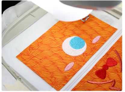
Zipper pouch designs with stiff felt pieces have dielines to show you where to place the felt pieces. This is to ensure that they are positioned perfectly after you turn the design right side out.
